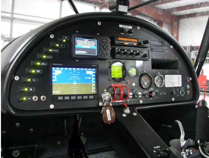
Latest panel showing optional Dynon D -100 EFIS and TL Electronics EMS systems
