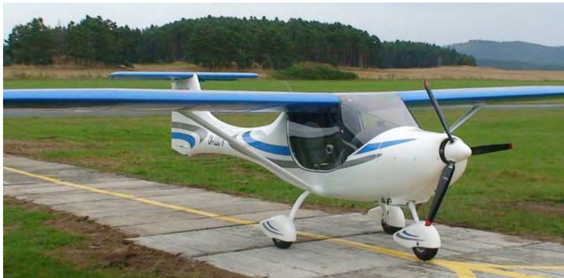
Allegro 2007 with latest low drag cowl – Note lack of opening for radiator – air is now drawn in around spinner and exits behind nose leg
