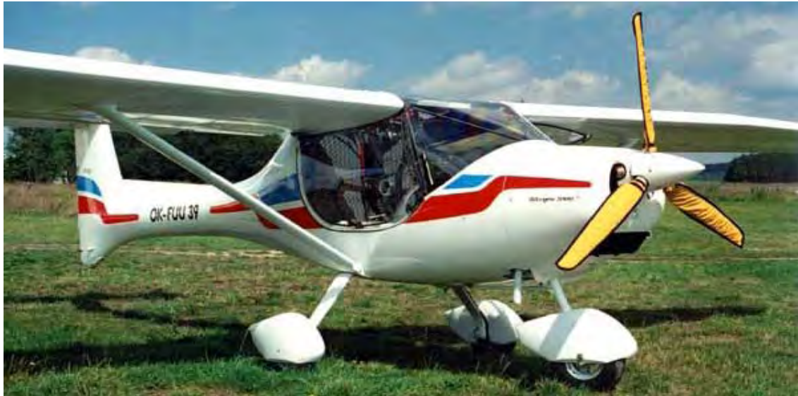
An earlier development aircraft showing old type engine cowl with external radiator (now internal for low drag)
