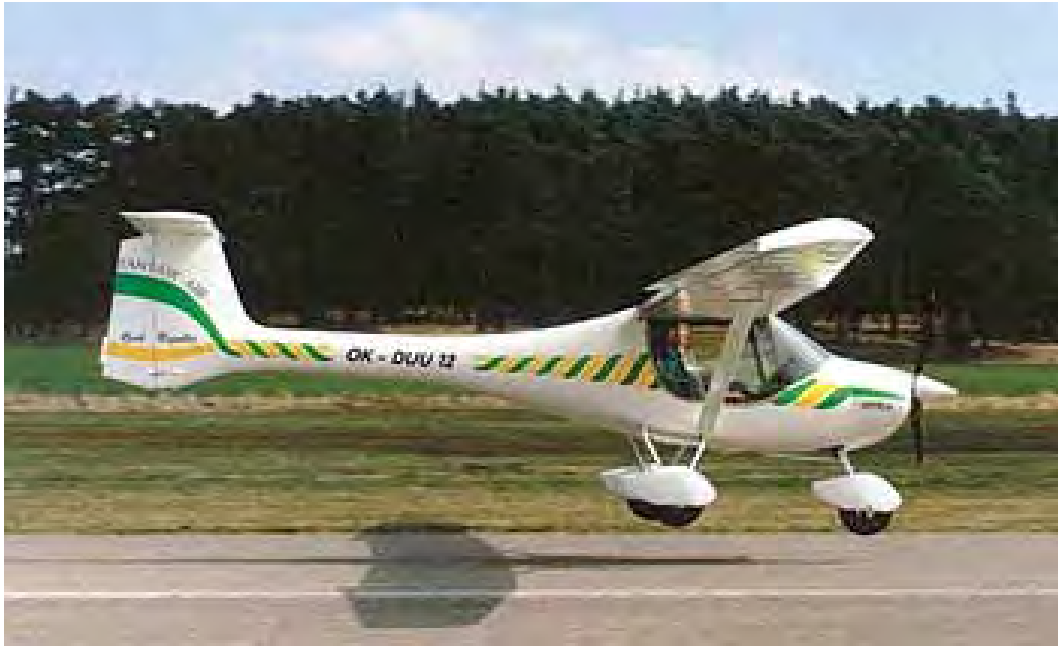
A very early Allegro with old type tubular main landing gear – now replaced with ultra tough Kevlar/Carbon composite
