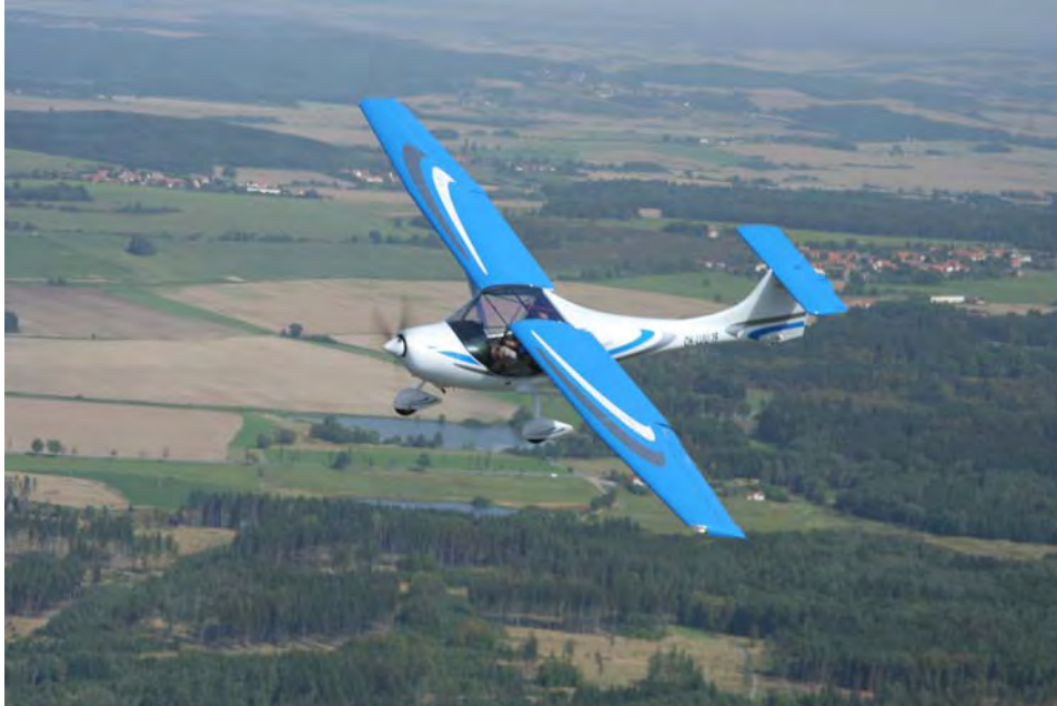
New 2007 Allegro showing Lexan roof panel that gives great visibility in tight turns and the circuit
