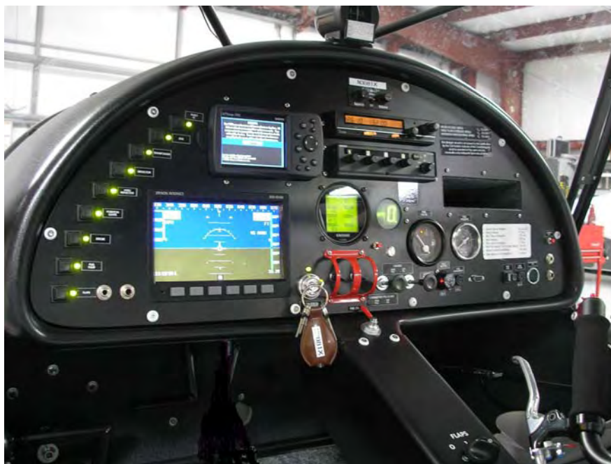
Latest panel showing optional Dynon D -100 EFIS and TL Electronics EMS systems
