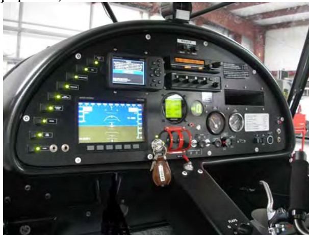
Dynon unit shown above - Flight Box has analogue type dials
