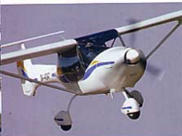
Owners can opt for two long-range wing tanks, gravity feeding fuel into the main tank, increasing capacity to 105 litres.
